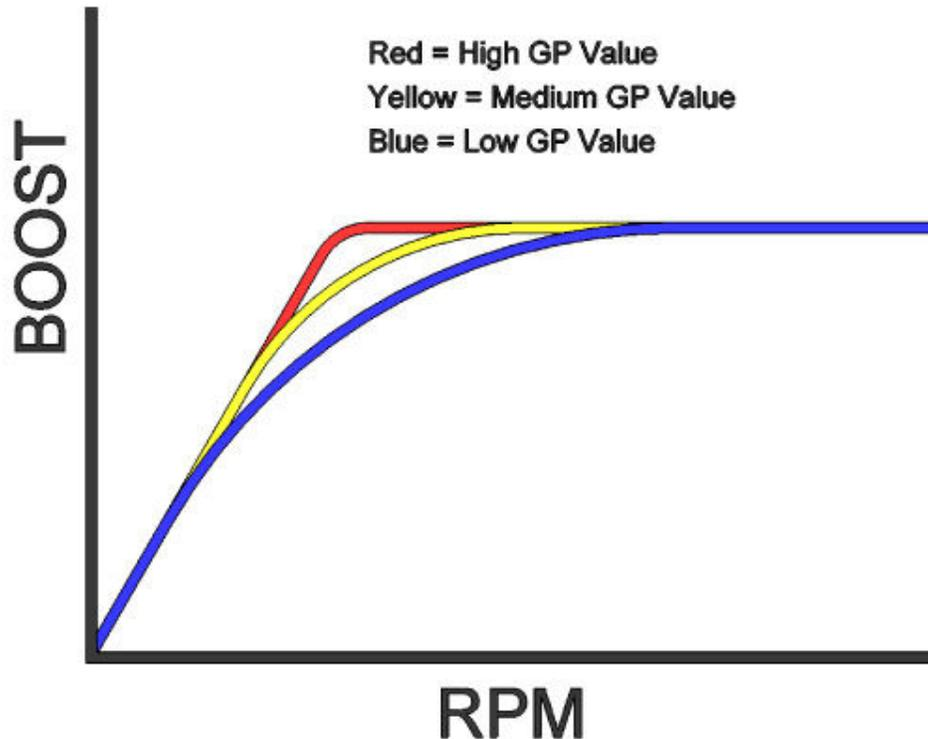
The Turbosmart manual boost controller range has an in built gate system which is set at 3 PSI. This means that below 3 PSI, the controller will clamp the signal to the wastegate, keeping it closed. If an undesirable boost spike occurs, removing the gate system by removing the ball and spring can eliminate the spike. Note: This modification is only required in a minimal number of applications.
