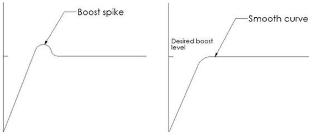
The Turbosmart e-Boost boost controller range has a gate pressure function that allows the user to choose what pressure the controller will allow boost pressure to reach the actuator. Setting the gate pressure at the optimum level will result in the best boost response from the turbo system. Set the gate
